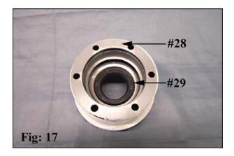
Next take #28 bearing housing (SC 2101) (Fig: 17) place it, machined end up on hand arbor press. Take #29 bearing housing seal (SL 1101) and lube outside circumference with WD-40. Align with seal bore in bearing housing install, spring side down (i.e. towards front of pump) visually inspect that seal is completely seated against seal bore shoulder.
